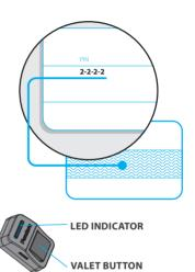
• ENTER THE THIRD DIGIT • Press the VALET button a number of times, equals to the third digit. Pauses between presses should not exceed 1 second. Each pressing will be confirmed with an orange LED indicator flash. A pause for more than 1 second and a red LED indicator flash confirm the input of the third digit. Then you can enter the next digit.
